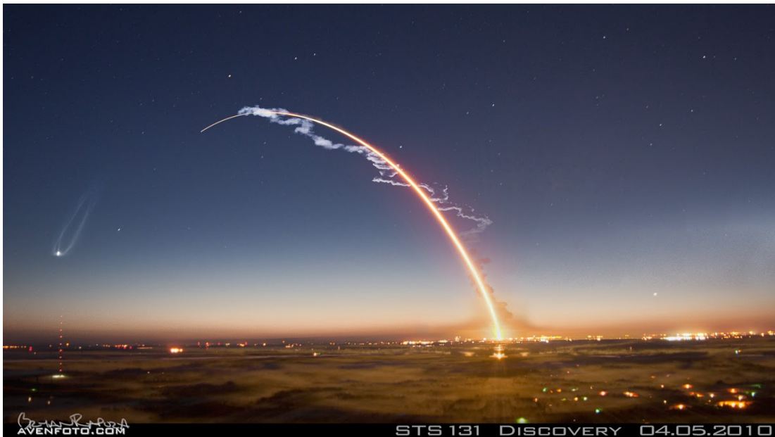
Plume affected by windshear as windspeed differs at various heights.
